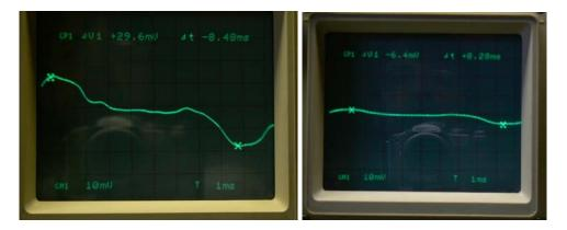
The example is fairly simple, illustrating mutual coupling between two transformers. The output transformer is terminated with an 8 ohm load and the power supply transformer is loaded only by filament current.) Voltage magnitudes are not that important however the *ratio* of improvement IS important. Coupling was reduced by 14 dB in this experiment.
