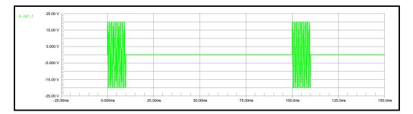
The audio generator is turned "on" for about 10 milliseconds every 100 milliseconds as can be determined by examining the waveform.
