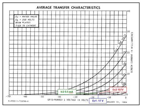
We now have all of the information required to design a voltage divider network for biasing the screen grid. The method discussed in Chapter 8.25 can be used, using the schematic below:
