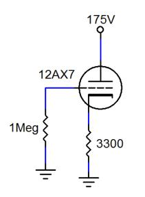
In this simple circuit, the cathode resistor is the component that determines plate current (lb), the grid resistor as noted previously is not particularly critical (47k to 1.0 Meg). The plate resistor will be selected to obtain the required gain and plate voltage for the tube. This part is not shown in these schematics and will be discussed later.
