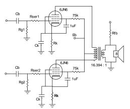
Note that the screen grids have been "bypassed" by connecting a capacitor between screen grid and cathode of both tubes. The capacitor provides a low impedance path from screen grid to cathode - if this isn't provided, the screen grid will behave like a smaller version of the plate, it will dissipate not only the bias voltage and current but the signal power will be added to the quiescent dissipation. Performance will be degraded and so will reliability.
