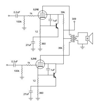
Note that the above schematic is an example of the bias feedback technique described - it's not intended to be a functional circuit to be copied and used in any arbitrarily selected amplifier.
