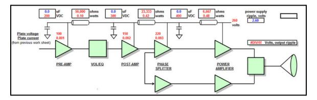
Error messages on the spreadsheet are a result of insufficient data entries. The object of this spreadsheet is to calculate the values and power ratings of the stage de-coupling resistors and allow the user to determine the value of de-
