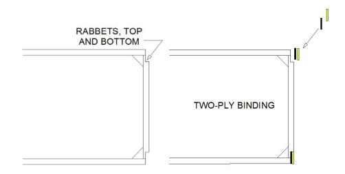
As shown in the second sketch, the binding is glued into the rabbets at the top and bottom of the guitar. The thickness of the individual binding strips is determined by the desired number of plies and the rabbet dimensions.
