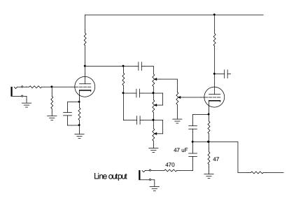
In order to avoid drilling a hole in the chassis of the amplifier (and to allow restoration to original configuration, if desired), the line output is usually wired to an input jack that is not normally used. It's helpful to mark this jack, even if the label is no more than a hand-written scrap of paper, taped near the jack.
