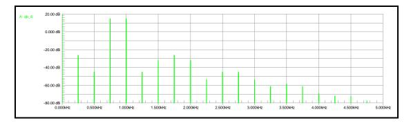
There is significantly more distortion in this simulation. In fact, if we were to calculate the difference between the two cases, we'd find that the first simulation had a distortion of about 1.6 % while the second case distortion was around 7.7 %, that's very significant ! So we were able to achieve an improvement in distortion of about 5 : 1 by increasing the power dissipation by a factor of 10. That's not a bad tradeoff.
