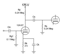
If all component values in the above schematic are known, the tables can be useful to approximate voltage gain. Conversely, knowing the gain required for a specific application, one can select a set of component values from tabulated data that will provide the voltage gain and output voltage swing. These tabulations were published many years ago, when vacuum tubes were of consistent performance. The tables may not provide accurate performance when used with currently produced devices.
