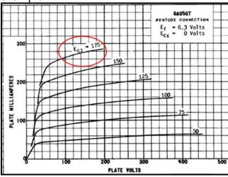
For this particular tube type, the manufacturer plotted screen grid bias voltages from 50 to 175 volts. I would take 175 volts as the maximum allowable screen grid voltage for this tube.
