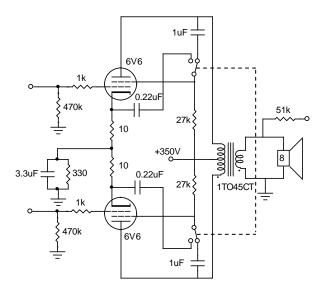
The screen grid bias will not change when switching modes. This configuration provides a power reduction from around 18 watts down to about 3 watts. (Recall that we normally consider capacitors to have zero impedance when considering signal conditions in the amplifier chain.)
