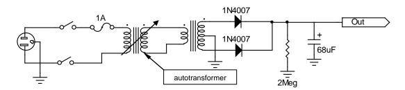
Autotransformers function **ONLY** with alternating current (A.C.) - never connect an autotransformer input to any circuit other than the household "line" voltage outlet. Always provide protection for excessive current draw (as in the accidental "short circuit"), to prevent this costly part from being destroyed by a wiring error or the like, if the autotransformer is not fuse-protected.
