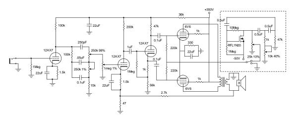
Here's the same Princeton circuit as above with a tremolo circuit added:
