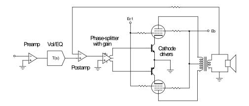
The control grids of the output tubes are effectively "grounded" through the control grid power supply. The cathodes are the "inputs" and the plates are still the output terminals. Note the use of negative feedback, from the speaker terminals back to the post amplifier that follows the volume/EQ control circuits.
