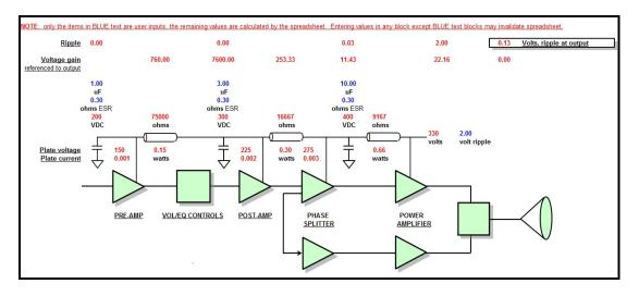
The user is required to entire a value for ripple voltage (obtained from the percentage ripple in the power supply spreadsheet. To use the ripple voltage from the spreadsheet, which is percentage, divide the percent ripple by 100 and multiply the result by the power supply voltage:
