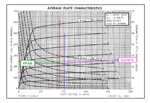
Now make a line at the Imax selected value of 230 mA. From the intersection of the Imax line with the two plate voltage lines, we can estimate a value of screen bias voltage, Ic2, at about 106 - 108 volts. This value should be adequate for either plate voltage application.
