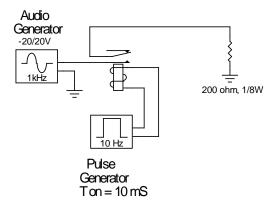
The audio generator is the test source and is adjusted to provide the output signal frequency and desired level. In series with the audio generator is a relay (either mechanical or a solid-state switch) that can be opened and closed by another generator (a square wave generator is best but not absolutely necessary).
