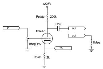
A computer simulation of this circuit indicated a voltage gain of around 35. The gain can be adjusted by varying the plate resistance if closer agreement is required. If an amplifier, when tested, exhibits low overall gain and the feedback gain (all of the gain in the stages that follow the post amplifier) is correct, then this stage would be the obvious place to make gain adjustments.
