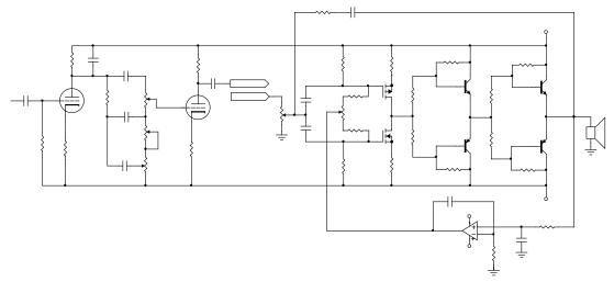
The ubiquitous 12AX7 front end was intended to be operated from the transistor power supplies of about +48 and -48 volts. This amplifier was intended to produce an output power level of 100 watts. I did make some experiments by "breadboarding" the tube part of the design, which is a configuration based on almost all vacuum tube amplifiers, regardless of manufacturer.
