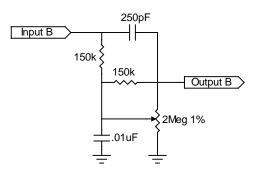
Here's another variation on the single-knob tone control, input impedance is about 30k when terminated in 1 Megohm. That's a little low for most preamps to
