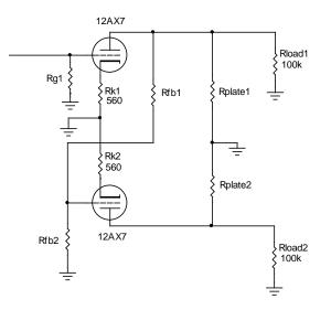
Now that we know the value of the cathode resistors and given a desired voltage gain value of Av = 10, we can re-arrange the expression for gain to read
