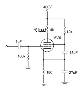
Assume that we now remove the 6V6 from its socket and replace it with a 6L6 and then a 6JN6, measuring the circuit performance for each tube and then summarizing.
