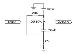
There are many variations in tone control configuration. My personal preference has always been the circuit used in post-1960 Fender amplifiers. It seems to have the most flexibility, although parts count is higher than other tone controls.
