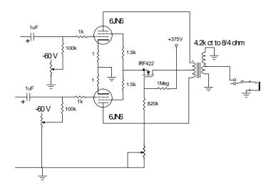
A high voltage MOSFET (heat-sunk to the amplifier chassis), referenced to an adjustable voltage divider, provides screen grid bias for the output tubes. The values selected gave an output power adjustment from about 25 to 45 watts, and the ability to achieve intentional power tube non-linearity as previously mentioned.
