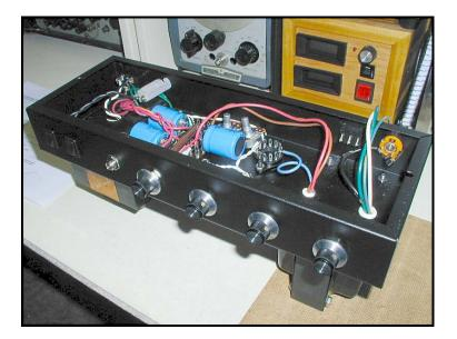
As we progressed through the various design exercises, we collected a number of individual circuits for each function in the amplifier chain. Except for the bias de-coupling circuits, and the high voltage supply line that connects the circuits, here's the signal chain, from preamplifier to speaker, for the medium power, fourtube amplifier.
