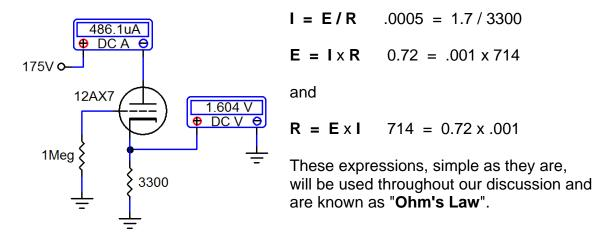
Note that many of the approximations that we use and the graphical means of extracting information from plate curves result in slight errors from the design values. Add the fact that we use "standard" resistor values rather than calculated values (and that those resistance values have practical tolerances) and *it should be apparent that there will be slight errors between calculations and measurements.*
