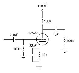
A computer simulation of the above circuit confirmed the gain of 46 in the table. If it were critical to obtain a voltage gain of 50 for the load and plate resistances in the previous example, one might increase the supply voltage up to 300 volts, as suggested by the tabulated component and performance values.
