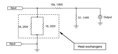
The output attenuator is configured to suit instrumentation with an input impedance of 50 ohms. If other impedances are desired (600 ohms is another "standard") then the 15k and 51 ohm resistors can be scaled by the ratio:
