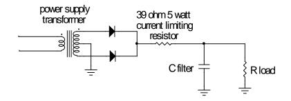
The diodes can be selected by their minimum PIV rating. PIV means "peak inverse voltage" and the rating must be greater than the peak voltage for the transformer. For the above example, the peak voltage is twice the peak voltage of the individual windings and is given by
