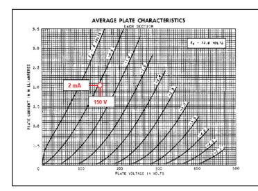
Examining the gate voltage curves (Ec), the gate voltage required to produce 2 mA current at 150 volts is about -0.5 volts.
