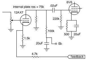
There are *three* resistors now that make up the plate load, the internal resistance of about 75k, the 100k plate resistor and the 220k grid resistor of the following stage. The effective plate load is
