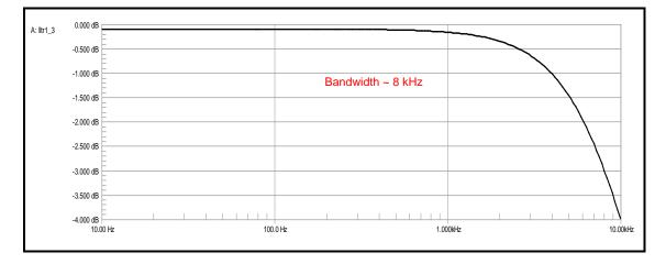
And if we double the length of the cable, the frequency response is degraded by the ratio of the two cable lengths:
