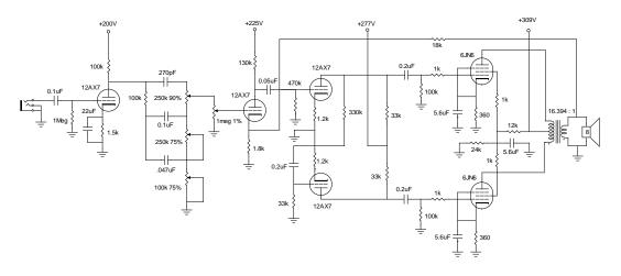
Some of the coupling (blocking) capacitor values differ from those shown in the chapters discussing the design of the individual circuits. When the entire amplifier is assembled (at least schematically) the parallel load resistances of each stage becomes easier to determine and new values of capacitance determined.
