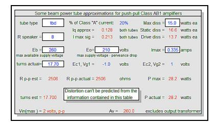
This looks impressive, the predicted output power is 28.2 watts, instead of the 15 watts we're trying to obtain! There are some problems, however... Look at the predictions of plate current, at the top of the spreadsheet. The two parameters "Iq approx" and "I max sig" both exceed our allowable power supply current of 100 mA. (Iq is the quiescent current and I max sig is the current at the maximum output power.)
