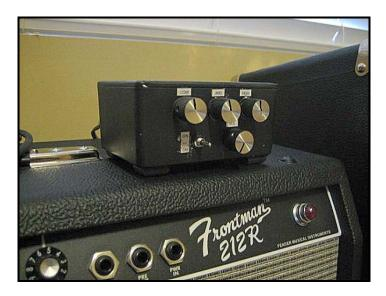
A preamplifier like this one is a useful addition to one's collection of cables, instruments, microphones and tools and can be built compactly enough to fit in a guitar case (or in the bottom of a combo amplifier). Note that the output is high impedance, however, and therefore long cables from the preamplifier are not recommended.
