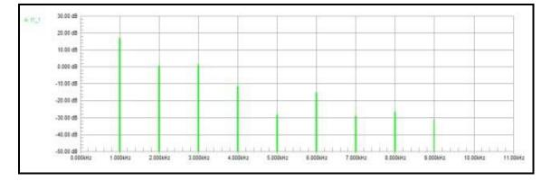
Now here's a spectral plot of a push-pull amplifier, like all of the ones in current usage. The fundamental signal is visible at the left and, as above, the other lines to the right are harmonics. BUT, note that the even order harmonics are much lower than the fundamental signal frequency and also all of the odd order harmonics. This is a computer simulation of a Fender "Princeton" amplifier:
