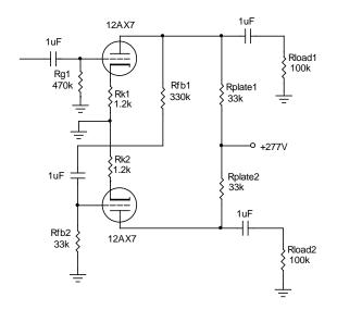
Running the circuit simulation a second time, using cathode resistor values of 1.5k instead of 1.2k predicted a voltage gain of 10.2. Note that the phase splitter will normally be inside the negative feedback loop so the gain of all stages within the loop will be externally established.
