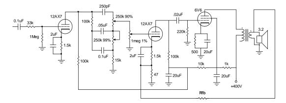
This small, Class "A" amplifier has a feedback network consisting of a single resistor (Rfb) connecting the output of the amplifier (speaker terminal) to the cathode of the post amplifier stage following the preamplifier and EQ/volume control. The location of the feedback "input" signal is important; it needs to be far enough "back" in the signal chain so as to affect most of the components in the chain.
