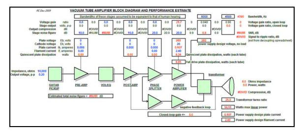
Note that there are some error messages displayed on the spreadsheet, these are a result of incomplete data entry. They will disappear as we gradually add the remaining data. Also note that all of the performance characteristics of the output stage already exist on the spreadsheet, they are automatically transferred, as the information on the power stage spreadsheet is updated.
