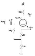
Note that the grid resistor is returned to a point between the two cathode resistors of 250 ohms and 20k. This establishes the bias condition of the phase splitter tube; the effective cathode bias resistance is 250 ohms NOT the series combination of 250 plus 20k. If the grid resistor were returned to ground through the 1 Megohm resistor, the cathode bias resistance would be 20,250 ohms and
