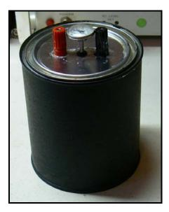
This is another variation of the high power load, this one is rated at 25 watts RMS continuously. Two 25 watt 16 ohm resistors, wired in parallel, are "sandwiched" between aluminum heat exchangers. Connected to the resulting 8 ohm load is an attenuator and a "BNC" connector (normally used for precision test equipment).
