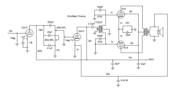
The modification was fun, informative and successful. The measured output power was about 12 watts at 5% distortion. Computer circuit simulations suggest that the output stage is capable of almost 20 watts (if cathode bias resistors are eliminated and a negative voltage is used to bias the grids of the output tubes, as in the Fender "Deluxe Reverb"). It is unlikely that the original power supply transformer or output transformer would last long at that power level, however.
