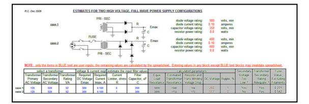
If we look at some of the information in the upper right corner, the critical component *selection* criteria are denoted. We're interested only in case 1 and we can determine that the two rectifier diodes required need to be rated at 900 volts minimum and 0.1 amperes minimum. The filter capacitor, 200 uF minimum, needs to be rated at least 350 volts, as shown. This is our first iteration of the power supply design and, to me, it looks pretty good, so we'll move on to the next step.
