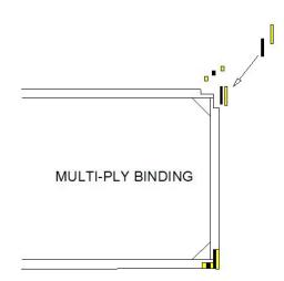
By making a second, shallow pass of the router and using two different thicknesses of binding, a wide decorative pattern can be achieved. A single router pass would cut through the side and into the lining, not a desirable situation. This is the technique employed on the 1976 Ovation illustrated at the beginning of this chapter. (The Ovation has the widest binding of any of my guitars, including the L-5 and the Golden Eagle.)
