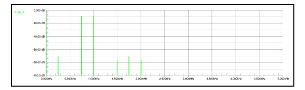
Very little difference is noted in the spectrum of the phase-splitter but then *this phase splitter has no gain*, and in fact can have a fair amount of loss, depending on the configuration. These simulations were performed on a phase-splitter that had 3 dB of loss.
