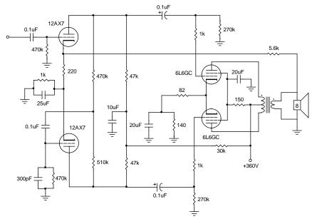
The circuit is conventional in most regards but has some subtleties that are slightly more sophisticated than many amplifiers available at the time (e.g. Fender, Gibson). The conservative attitude of the original designers is apparent in the inclusion of multiple cathode bias resistors. Cathode resistors provide series feedback and enhance bias stability.
