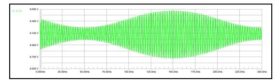
All that's needed to produce this effect is a low-frequency oscillator, whose frequency and amplitude are variable and the proper place in the amplifier chain to insert the signal. We want to use the output voltage from the low-frequency generator to vary the bias at a point in the chain that will have a significant effect on the signal level.
