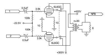
The double-pole-double-throw (DPDT) switch connects the screen grid either to a separate screen bias voltage or directly to the plates of the two tubes. The output power varies from around 30 watts to about 5 watts in the two switched states of operation above.
