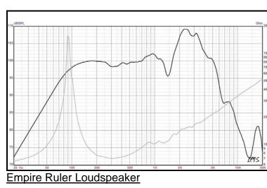
Looking at both performance curves carefully, Tal observes that "his" loudspeaker has higher SPL (it's louder) but less bandwidth (total frequency response) than the "Empire". He makes what *he* believes is a reasonable assumption: that the *total sound pressure level* each loudspeaker projects is actually about the same. He believes the difference is in the power *distribution* across the frequency range.
