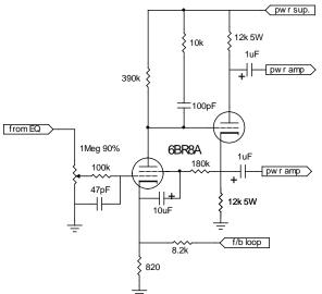
The conservative choice would be the phase-splitter with gain, since the pentode circuit hasn't been tried in a combo amplifier (at least, not by me). Guitar amplifiers universally use the dual triode configuration - high-fidelity amplifiers
