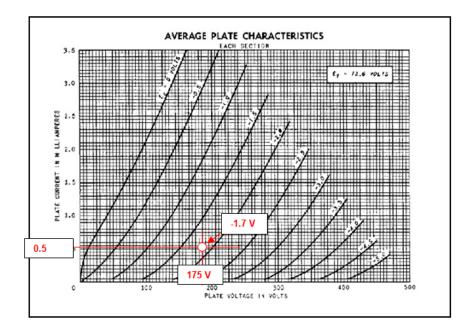
Examining the point on the curve representing 0.5 milliamps and 175 volts we can then estimate (from the curves of control grid voltages, Ec1) that the approximate grid voltage required to produce a current flow of 0.5 milliamps at a plate voltage of 175 is about -1.7 volts.
