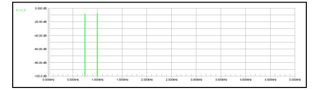
Here's a spectral representation of two pure (unmodulated) sine waves:
