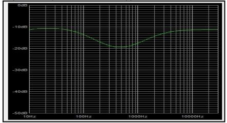
Response with bass at "10", treble at "0" results in treble cut of about 10 dB:
