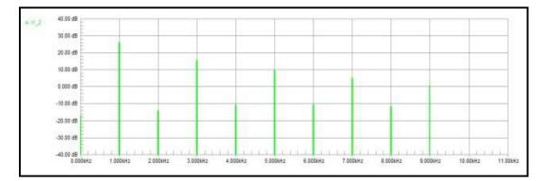
Note: this configuration suppresses the even order harmonics that are generated by the output tubes, NOT distortion that has been previously introduced further back in the circuit (including intentional distortion).
