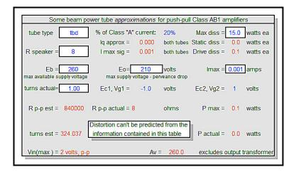
Now comes the iterative part of the power stage design. We need to find the right tube and the right output transformer that can produce 15 watts of output power given the supply voltage and current restraints that we have to work with.
