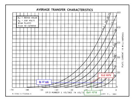
Noting that the control grid voltage is -17 volts, we move on to the next set of curves. We can draw two lines representing the control grid 1 voltage and the screen grid voltage of 107 volts, then find the screen current from the left vertical axis of the curve:
