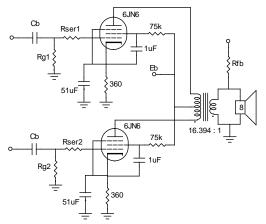
In past days, as we've noted previously, the practice was to connect the two cathodes together and then connect them to ground through a resistor of 1/2 the resistance of a single cathode resistor. This allows higher gain at the expense of bias stability. A good compromise might be to use three resistors, as shown in the circuit below, for cathode bias:
