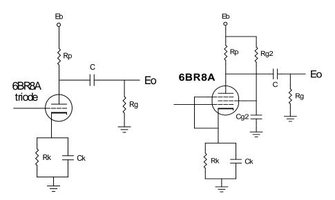
(Remember that this is a dual tube - both the triode and the pentode are in the same package.) The values in the tables are specific to the 7199 tube but I've also used the tabulations for the inexpensive 6BR8 tube. It's always wise to find tabulated data for the specific tube under consideration or design each section conventionally (graphically). If one has the time to breadboard the circuit, I'd suggest using the tabulated values and then optimizing the values at breadboard stage.
