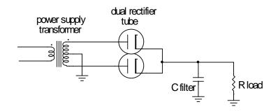
Avoiding reference to specific amplifiers, let's assign some values to the rectifier circuit. Assume that the RMS output voltage of the transformer is about 400 volts, center tapped (200 volts RMS at each "leg" of the transformer). The maximum, unloaded D.C. output voltage available will be:
