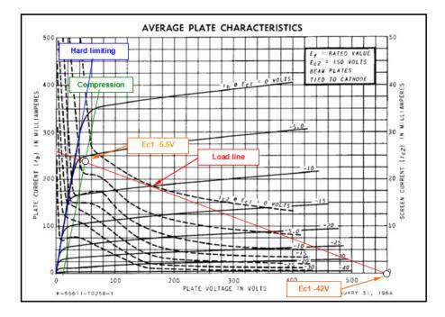
One can easily draw a line denoting the area where compression starts, by observing where the plate curves commence to deviate from a straight line. We can add a point to the load line (at Eb = 50 volts). Adding a point at the upper limit of 572 volts establishes the minimum and maximum limits of linear operation. We can also note that the grid voltage, Ec1, for these two conditions is -5.5 volts and -42 volts.
