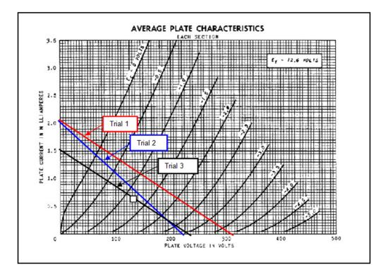
We can see that when the gate voltage is at -3 volts, the plate voltage probably cannot reach the supply voltage of 210 volts. Let's make one final revision and set the supply voltage (the maximum plate voltage) at 225 volts, then adjust the slope of the load line for a 150 volt plate variation when the grid voltage varies by 3 volts, call this "trial 3".
