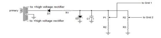
Note that the two diodes have markings that indicate specific polarization, as does the capacitor. These polarities must be observed when installing the components.
