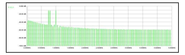
As more signals are added and the intervals between them decreased (such as would be the case in chords utilizing more than two or three notes) the distortion products increase and produce more audibly displeasing sounds. The obvious question is how to eliminate these undesirable products? That's not possible but there are ways to suppress them to a more tolerable level.
