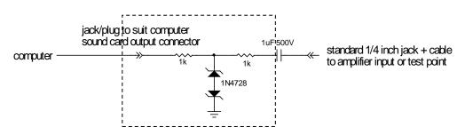
This circuit will protect the sound card from high DC voltages or AC voltages but the virtual signal generator shouldn't be intentionally applied to a test point where dangerous voltages may be present. Additionally, the virtual generator can't be used to drive low impedance loads. This will never present a problem when working on vacuum tube guitar amplifiers.
