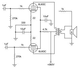
The value of the two un-bypassed resistors must not be too large or else gain will be lost. The advantage is the provision of *some* D.C. feedback so that unmatched output tubes will share current more equally than if a single cathode resistor, common to both cathodes, was used. (Design values will depend on the anticipated variation in output tube transconductance.)
