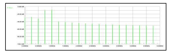
Where did all those other signals come from ? The other signals are harmonic and "intermodulation products" - they occur whenever signals are passed through a non-linear network (ALL amplifiers). What happens is that the 750 Hz
