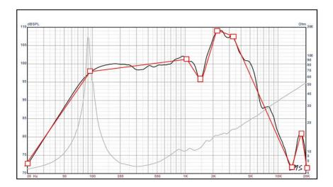
As in the first exercise, Tal normalized all of the sound pressure levels by subtracting the maximum SPL rating from the nine points shown on the above graph. The maximum SPL is 109 dB, so "109" is the value that must be subtracted from the other eight points on the curve.
