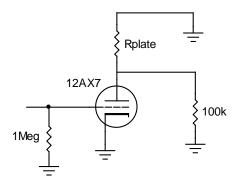
The total output load is the plate resistor in parallel with the 100k load resistance. Any value of plate resistance is going to make the total resistance lower than 100k. Let's look through the table of component values again, this time with the idea in mind that we need a total load resistance less than 100k.
