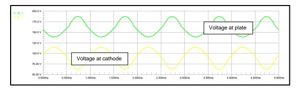
Since the output voltages from plate and cathode are connected to the following stages with capacitors, the DC component of the signal voltages is blocked - only the AC signals are passed to the next stage. The signals, as was desired, are of equal amplitude and 180 degrees out of phase (which means that if one signal is
