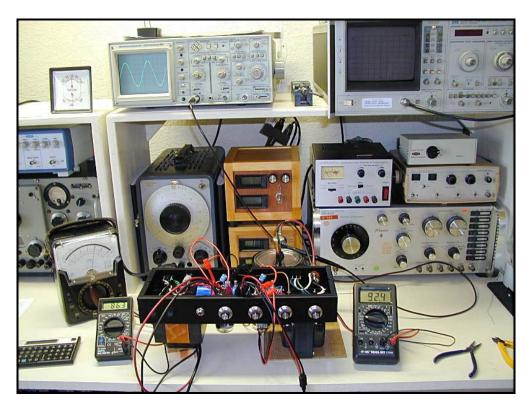
Two DMMs are measuring the voltage drop across 1 ohm resistors connected to the cathode of each output tube, the voltage (in millivolts) measured across a 1 ohm resistor is equal to the cathode current (in milliamperes). An analog voltmeter (the one with the "needle" on the left) is connected across the terminals of the "dummy load", measuring the A.C. RMS voltage from which the output power level can be determined.
