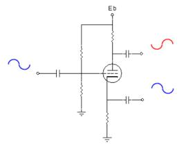
There are two types of phase shifters, differentiated by whether they have gain or not. The common configuration in smaller, low-power amplifiers is a phase shifter that has no gain – it simply divides the incoming signal into two signals and inverts the phase of one of them. This type always uses a single tube - or else one element of a dual triode - and examples of this are seen in amplifiers like the small Fenders (e.g. the Princeton mentioned above).
