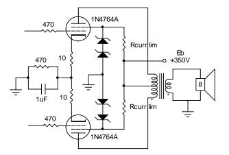
The current limiting resistors are chosen to operate the zener diodes at a safe dissipation, which is usually about 1/2 the maximum dissipation. For the above diodes, rated at 1 watt, we need to operate each diode at 500 milliwatts or 0.5 watts. The current required for this dissipation is given by
