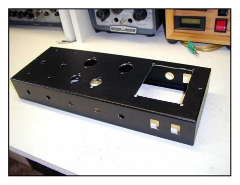
All of the work performed on this chassis can be accomplished in an afternoon with a drill press, the tools mentioned above and a "nibbler". It's even possible to do this work with a hand drill (drilling a sequence of holes that are almost tangent to one another, breaking out the waste material and then filing edges smooth) and I have often done so, when more suitable tools were lacking.
