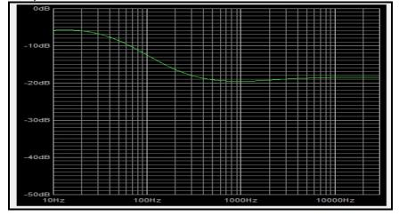
Response with bass at "0", treble at "10" results in bass cut of about 10 dB:
