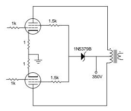
If the 1.5 k current limiting resistors were much larger in value, it would be wise to add a bypass capacitor between screen grids and cathodes. Note that the power rating of the zener should exceed the actual dissipation by a factor of 2. The dissipation is calculated as follows:
