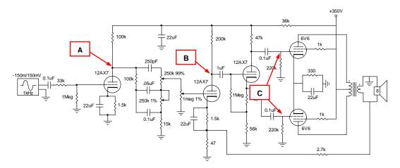
"A" and "B" are injection points to the plates of the preamplifier and post amplifier, respectively. Typical requirements of modulation injected at these points are that the output impedance of the modulator be five or ten times greater than the effective plate resistance (so that the stage gain is not degraded) and the peak-to-peak modulation current is adequate to cause a voltage change across the plate resistance that allows normal operation or near complete cut-off of the tube.
