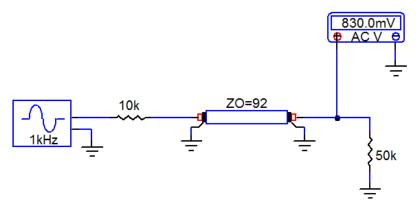
The schematic is a screen capture of a computer circuit analysis simulation. In circuit analysis, a signal generator (or a battery) is always assumed to be zero impedance so the series resistor of 10k ohms represents the source impedance (generator impedance of zero ohms + 10k ohms = 10k ohms). The output voltage of the signal generator has been fixed at 1 volt RMS in this example.
