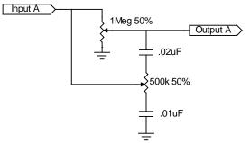
This is a tone control circuit from a Gibson amplifier of the same era, Model GA-79RTV. This circuit falls in between the Fender and Ampeg tone controls in complexity and provides acceptable performance for most pickups. The input impedance of this circuit is approximately 150k if terminated with 1 Megohm.
