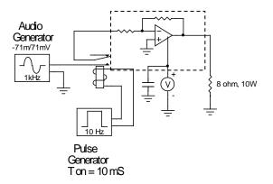
The amplifier under test is represented by the simple schematic within the dashed lines; it has a voltage gain of about 500. If the amplifier were driven by the audio generator in a steady-state condition (not pulsed), the 8 ohm output load would be required to absorb **80 WATTS**. The 10 watt resistor wouldn't last long at that level. But since the pulsed duty cycle is only 10%, the actual dissipation of the load is only **8 watts**. (The RMS power times the duty cycle.)
