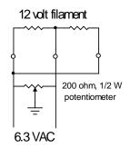
There are several more drastic "solutions" to the hum problem. Since the problem normally is caused by poor layout or poor grounding, these options won't help, as a rule. They have been used in the past for high-fidelity stero power amplifiers, where power supply noise needs to be some 100 dB below the signal, for example. The simplest option is to operate the filaments from a regulated D.C. voltage:
