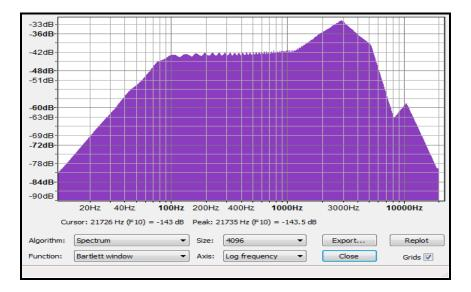
He then repeated the exercise, using the SPL curves from the "Empire Ruler" speaker that he is considering, first drawing straight lines to approximate sections of the SPL curve that are linear and using the intersections of the lines to define the points that will be used for equalization. After spending a few moments, Tal's results produce the following :
