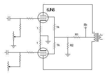
Eb = 305 volts Ec2 = 107 volts Ic2 = 0.5 mA or .0005 amperes
