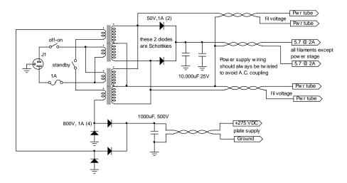
A few comments regarding the power supply: This concept can be extended to three transformers for greater voltage capability. Schottky rectifier diodes are required *in the filament circuit* to minimize voltage drop (about 0.3 volts for the Schottky diodes versus 0.8 volts for standard rectifiers). The above component values and ratings are minimum - substitutions of greater values and greater ratings are perfectly acceptable.
