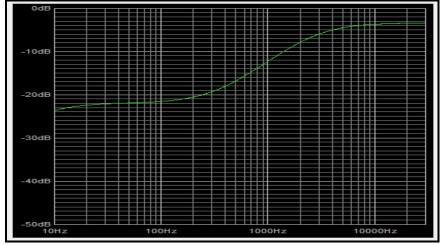
It is apparent that the adjustments are adequate for the typical requirement - the maximum loss is about the same as the specification and the connections are as described. The logarithmic response will be assured by selecting potentiometers that exhibit that characteristic. If a "mid" tone control is desired, it is usually linear response, not logarithmic.
