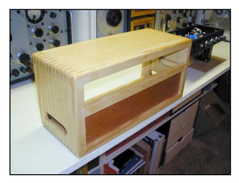
Note that to maintain the clean lines of the design, this cabinet has hand holes routed in the side instead of a standard handle secured to the top. (The hand holes also permit the circulation of cooling air within the cabinet.) The lower front panel of the enclosure is a small sheet of 1/4 inch mahogany plywood - the type is not critical.
